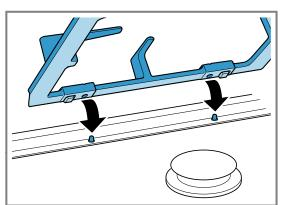
Place the cookware correctly on the pan supports. Never place the cookware directly on the burner. Always carefully remove the pan supports. When moving a pan support, the pan supports next to it may also move. **Tip:** You can remove the metal residue that remains when some items of cookware are moved on the pan support by cleaning it properly.
