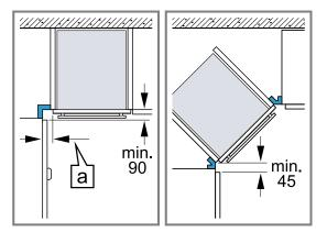
To ensure that the appliance door can be opened, you must take the minimum dimensions into consideration when installing in a corner. The dimension is dependent on the thickness of the unit front and the handle.
