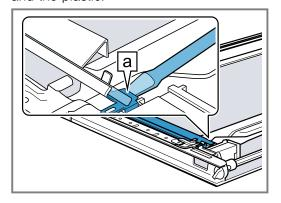
**6.** Use the screwdriver to lift 1 the reflector 1 until it disengages, then lift it up and pull it out 2.
