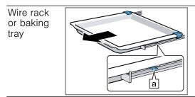
2. Hold the accessory on both sides in the area marked a and remove it.
