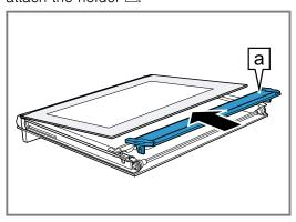
12. Insert the inner pane with the holder a into the opening.
