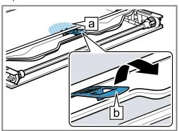
9. Lift the first and second intermediate panes from below 1) and remove them in the direction of the arrow 2.
