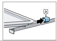
**5.** Push the accessory all the way in, making sure that it does not touch the appliance door.
