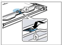
The retainer has been inserted.
