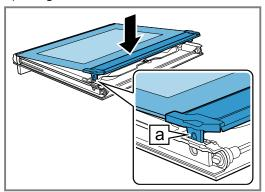
13. Screw both screws back in on the left and right of the appliance door.
