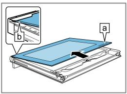
**11.** Carefully lift the inner pane upwards at an angle and attach the holder a.
