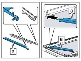
7. Insert the reflector and click it into place in the gap b.
