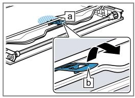
5. Lift the intermediate pane from below ① and remove it in the direction of the arrow 2.
