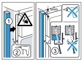
**9.** Open the appliance door slightly, then refit the panels and screw them in place, first at the top and then at the bottom.
