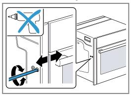
Turning the screws clockwise makes the gap larger Turning the screws anti-clockwise makes the gap smaller
