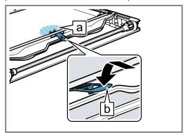
The retainer has been inserted.
