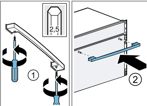
5. Tighten the screws until the door handle is secured.
