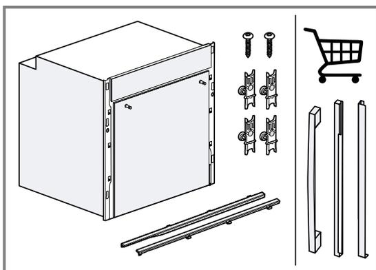
Depending on the appliance configuration, different handles and panels can be used. An example is shown in the picture.
