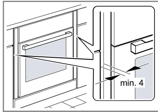
There must be an air gap of at least 4 mm between the appliance and adjacent unit fronts.
