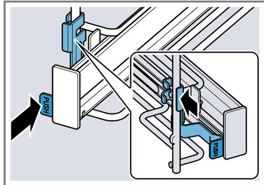
2. Press and hold **PUSH** ① and swing the rail outwards ② until the front retainer a is detached.
