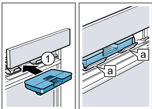
9. Slowly slide the control panel downwards and then push it away from you until it is closed completely.
