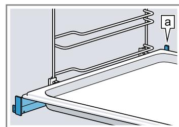
**Note:** The pull-out rails lock in place when they are fully pulled out. Gently push the pull-out rails back into the cooking compartment.
