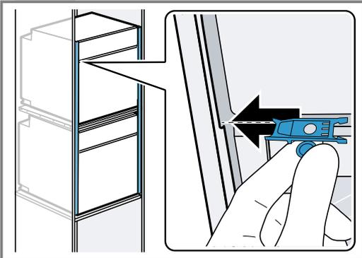
3. Turn the fastening element to the left or right to adjust the alignment of the panels.
