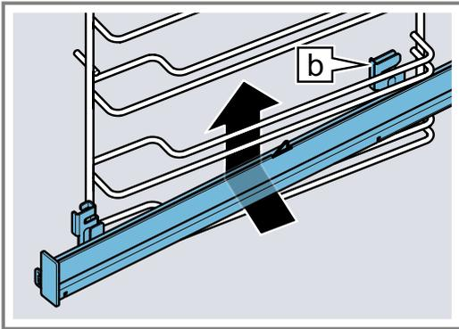
2. Guide the rail lengthways to the rear to the guide rods, and slide both retainers onto each lower rod. In doing so, use the rear retainer **b** to grip the vertical rod.
