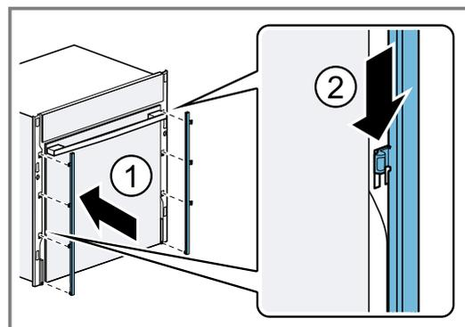
11. Push on the left- and right-hand panels at the height of the fastening elements until a clicking sound is heard.
