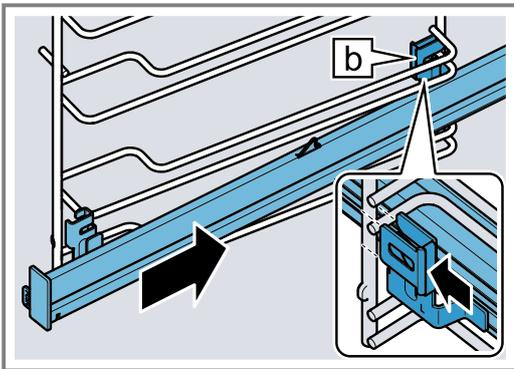
3. Press and hold **PUSH** **1** and swing the pull-out rail inwards **2** until the retainer **a** is attached in the lower rod.
