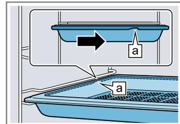
3. To place the accessory at shelf positions with pull-out rails, pull out the pull-out rails.
