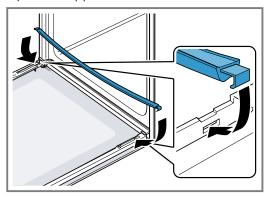
6. Note: When sliding the pane in, ensure that the glossy side of the pane is on the outside and the cut-outs on the left and right are at the top.
