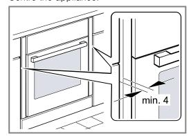
There must be an air gap of at least 4 mm between the appliance and adjacent unit fronts. **3.** Open the appliance door and unscrew the left and right-hand panels.
