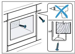
**6.** Refit the panels and screw them in place, first at the top and then at the bottom.
