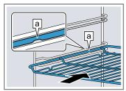
Tray E.g. universal pan or baking tray Slide the tray in with the sloping edge b towards the appliance door.
