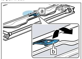
5. Lift the intermediate pane from below 10 and remove it in the direction of the arrow 2.
