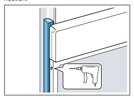
3. Secure the appliance using a suitable screw.
