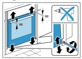
Turning the screws clockwise makes the gap smal-
