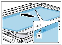
The arrow on the intermediate pane must line up with the arrow on the frame a.
