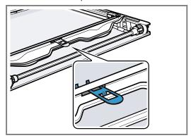
The retainer has been inserted.
