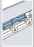
9. Slowly slide the control panel downwards and then push it away from you until it is closed completely.
