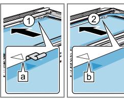
The arrow on the intermediate pane must line up with the arrow on the frame b.
