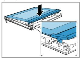
**9.** Screw both screws back in on the left and right of the appliance door.
