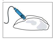
**Note:** If you want to turn the food, insert the meat probe into the side of the food so that it does not need to be removed when turning.
