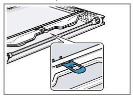
The retainer has been inserted.
