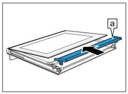
8. Insert the inner pane with the holder a into the opening.
