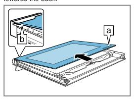
7. Carefully lift the inner pane upwards at an angle and attach the holder a.
