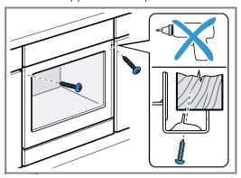
8. Open the appliance door slightly, then refit the panels and screw them in place, first at the top and then at the bottom.
