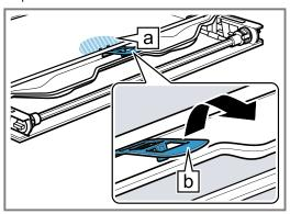
6. Lift the first and second intermediate panes from below 1 and remove them in the direction of the arrow (2)
