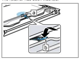
6. Place the inner pane onto the appliance door so that the number a is legible at the bottom right. Insert the inner pane into the fixing rail at an angle towards the back.
