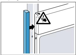
2. Pre-drill aluminium profiles to establish a screw connection.
