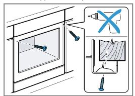
8. Open the appliance door slightly, then refit the panels and screw them in place, first at the top and then at the bottom.
