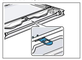
The retainer has been inserted.
