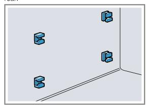
1. Hook the front retainers with the hook into the round hole at the top and set them at a slight angle  $^{\circ}$ .
