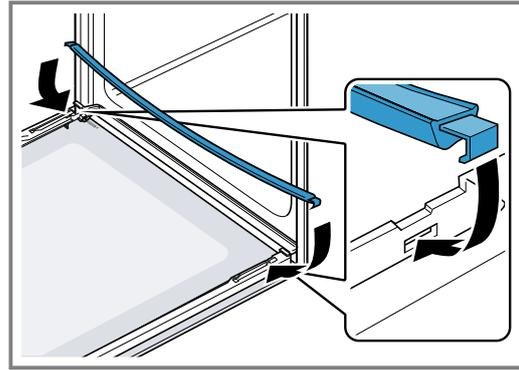
6. **Note:** When sliding the pane in, ensure that the glossy side of the pane is on the outside and the cut-outs on the left and right are at the top. Slide the inner pane into the left- and right-hand retainers **a**.
