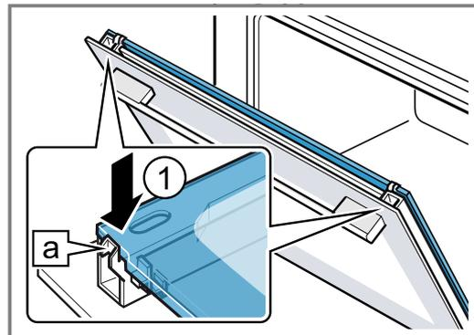
8. Put the door cover into position **1** and push down on it until you hear it click into place.
