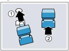
**3.** Hook the rear retainers with the hook into the top hole ① and push them into the bottom hole ②.
