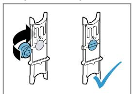
**2.** Hook in the fastening element at the bottom and press down at the top until it is in place.
