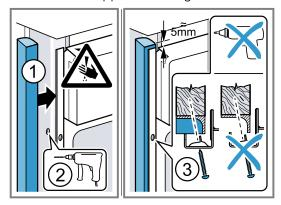
**Note:** The gap between the worktop and the appliance must not be sealed by additional strips.
