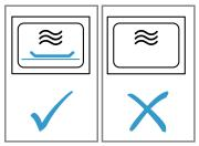
If you prepare microwave popcorn at a microwave power level that is too high, the door pane may crack due to overloading.
