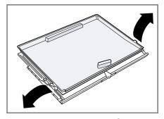
**4.** Lift the cover at the front ① and pull it out at the rear 2.
