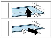
Press in the snap-in hooks on the side of the container 1 and remove the front from the container in a turning motion 2.
