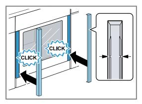
The arrow inside the panels must point upwards. Position the groove on the panels above the corresponding transverse rib on the red fastening part.
