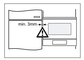
There must be an air gap of at least 3 mm between the appliance and adjacent unit fronts.
