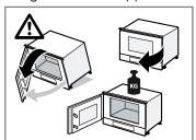
1. Open the appliance door 60° 10 and slide a fastening element directly above the control panel between the appliance door and the control panel 2.
