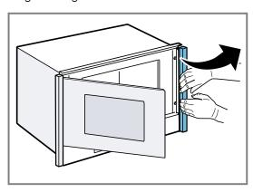
**4.** If the fastening elements have become loose when removing the panels, reattach them. Hook in the fastening element at the bottom and press down at the top until it is in place.
