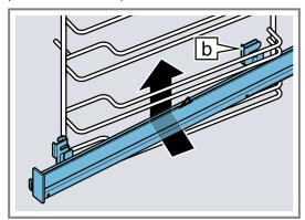
2. Guide the rail lengthways to the rear to the guide rods, and slide both retainers onto each lower rod. In doing so, use the rear retainer b to grip the vertical
