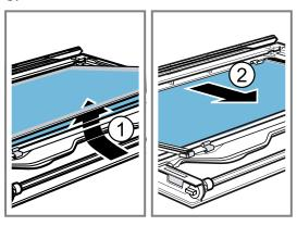
7. Remove the spacers a and seals for cleaning, if re-
