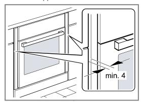
There must be an air gap of at least 4 mm between the appliance and adjacent unit fronts.
