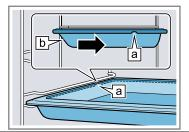
Place the accessories on the inserted pull-out rails.
