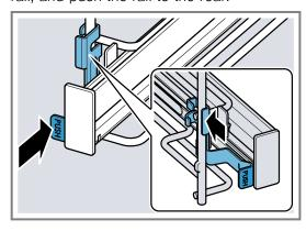
2. Press and hold **PUSH** ① and swing the rail outwards ② until the front retainer ⓐ is detached.
