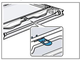
The retainer has been inserted.
