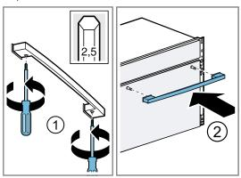
**5.** Tighten the screws until the door handle is secured.
