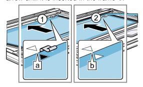
The arrow on the intermediate pane must line up with the arrow on the frame **b**.
