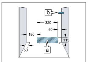
For appliances that have a hinged switch panel, make sure that the switch panel does not hit adjacent kitchen units when you open
