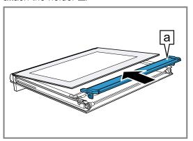
**9.** Insert the inner pane with the holder a into the opening.
