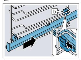
3. Press and hold **PUSH** ① and swing the pull-out rail inwards 2 until the retainer a is attached in the lower rod.
