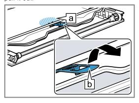
6. Lift the first and second intermediate panes from below 1) and remove them in the direction of the arrow
