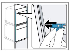
**3.** Turn the fastening element to the left or right to adjust the alignment of the panels.
