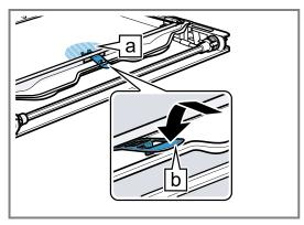
7. Place the inner pane onto the appliance door so that the number @ is legible at the bottom right. Insert the inner pane into the fixing rail b at an angle towards the back.
