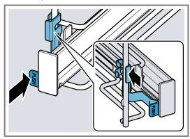
2. Press and hold **PUSH** ① and swing the rail outwards ② until the front retainer ② is detached.
