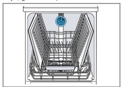
Arrange max. 2 baking sheets and 2 grilles as shown to ensure that the spray iet can reach all parts.
