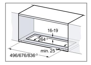
Make the cut-out for the exhaust air pipe either above the fitted unit or behind the fitted unit above the appliance.
