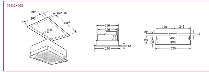
Measurements in mm. The line drawings featured in this brochure are provided as a guide to general dimensions only and are subject to amendment without prior notice For full dimensional and installation details please refer to the documentation supplied with the appliance
