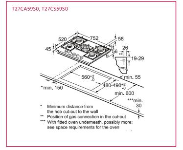
Measurements in mm. The line drawings featured in this brochure are provided as a guide to general dimensions only and are subject to amendment without prior notice. For full dimensional and installation details please refer to the documentation supplied with the appliance.
