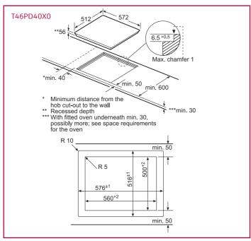
Measurements in mm. The line drawings featured in this brochure are provided as a guide to general dimensions only and are subject to amendment without prior notice. For full dimensional and installation details please refer to the documentation supplied with the appliance.
