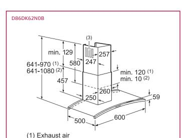
exhaust air slot facing downwards
