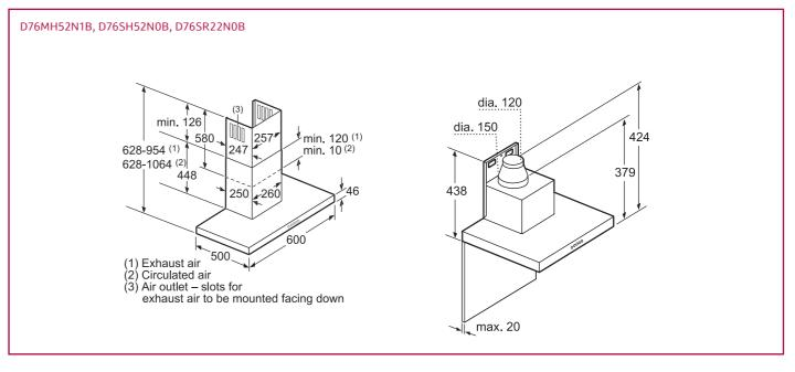
Measurements in mm. The line drawings featured in this brochure are provided as a guide to general dimensions only and are subject to amendment without prior notice. For full dimensional and installation details please refer to the documentation supplied with the appliance.
