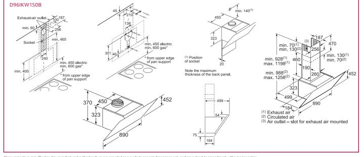
Measurements in mm. The line drawings featured in this brochure are provided as a guide to general dimensions only and are subject to amendment without prior notice For full dimensional and installation details please refer to the documentation supplied with the appliance.
