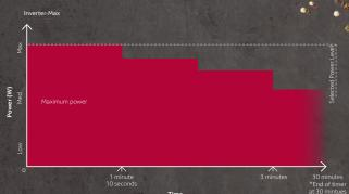
Inverter: Automatically manages the power levels during the cooking time
