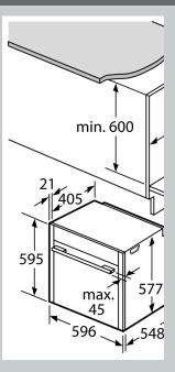
If the appliance will be a hob, the following w (including substructur must be taken into ac
