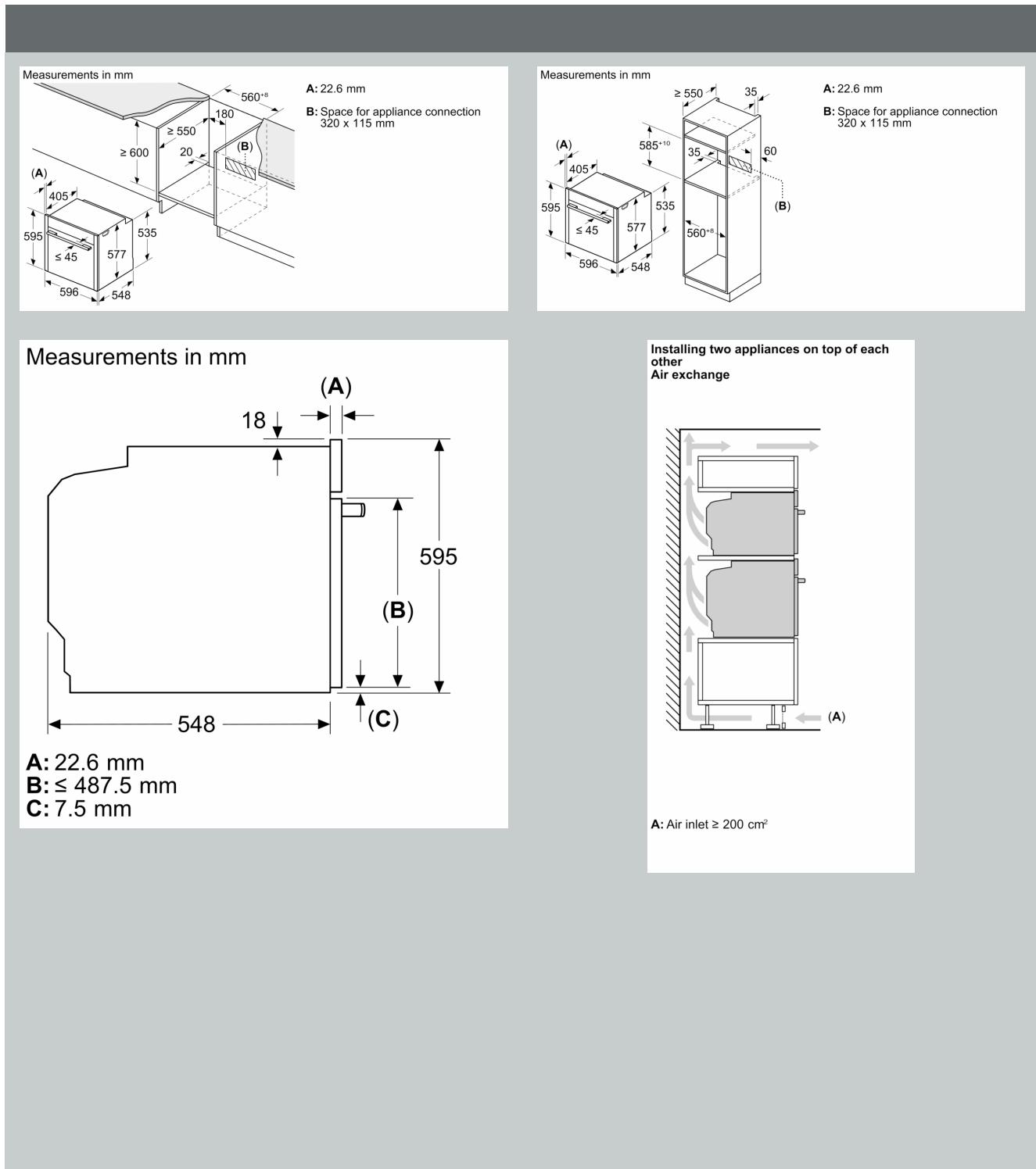
If the appliance will be installed underneath a hob, the following worktop thicknesses (including substructure if necessary) must be taken into account.
