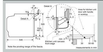
If the appliance will be installed underneath a hob, the following worktop thicknesses (including substructure if necessary) must be taken into account.
