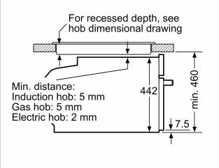
If the compact appliance will be installed underneath a hob, the following worktop thicknesses (including substructure if necessary) must be taken into acccount.
