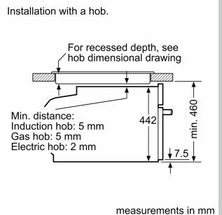
If the compact appliance will be installed underneath a hob, the following worktop thicknesses (including substructure if necessary) must be taken into account.
