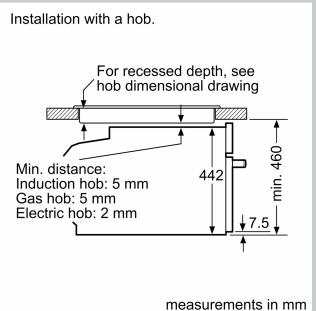
If the compact appliance will be installed underneath a hob, the following worktop thicknesses (including substructure if necessary) must be taken into account.
