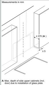
Appliance must be installed before upper cabinets, if these are deeper than 370 mm
