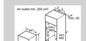
Ventilation space in the base min. 200 cm<sup>2</sup> measurements in mm
