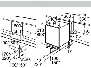
\* variable base/substructure height
