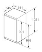
measurements in mm
