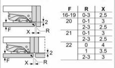
The gap dimensions recommended in the table must be adhered to in order to ensure that appliance doors do not collide with anything when they are opened, and to avoid causing damage to kitchen units.
