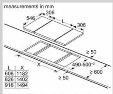
When installing two Domino units right next to a hob, two assembly kits (Z9914X0) are required.
