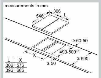
When installing two or more Domino units side-by-side, one or more assembly kits are required (2 units = 1 assembly kit; 3 units = 2 assembly kits, etc.).
