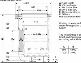
Ducting kit available for ≥ 600 mm depth worktops and up to 960 mm height
