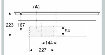
measurements in mm Front view – unit cut-out for unducted recirculation
