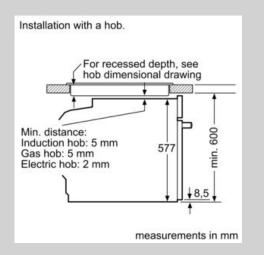
If the appliance will be installed underneath a hob, the following worktop thicknesses (including substructure if necessary) must be taken into account.
