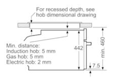
measurements in mm
