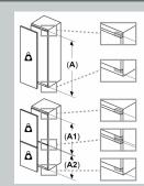
Fitted unit fronts that exceed the permissible weight may cause damage and result in functional impairment of the hinges  $\mathring{\Delta}$  Weight  $\mathring{\Delta}$ : Appliance door height including hinges in mm
