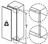
Fitted kitchen unit doors that exceed the permissible weight may cause damage and result in functional impairment of the hinges.
