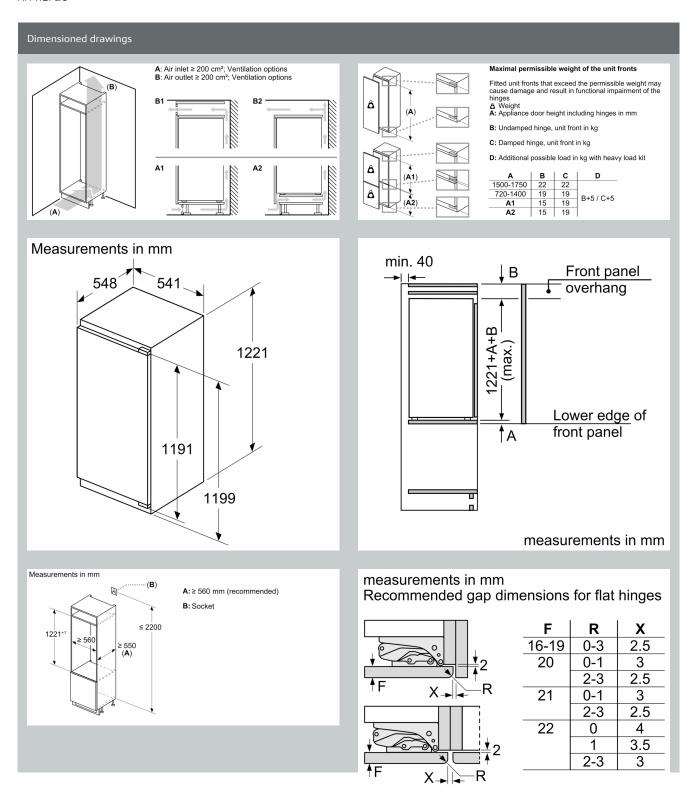
The gap dimensions recommended in the table must be adhered to in order to ensure that appliance doors do not collide with anything when they are opened, and to avoid causing damage to kitchen units.
