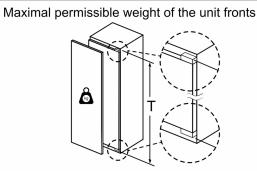
Fitted kitchen unit doors that exceed the permissible weight may cause damage and result in functional impairment of the hinges.
