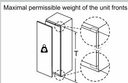
Fitted kitchen unit doors that exceed the permissible weight may cause damage and result in functional impairment of the hinges.
