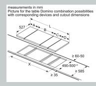
If two or more elements are installed right next to one another, one or several installation kits are required (2 elements 1 installation kit, 3 elements 2 installation kit, 3.
